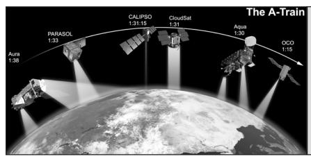
FIGURE 1: This graphic (not to scale) depicts the satellites that make up the Afternoon Constellation—"The A-Train". Listed under each satellite's name is its equator crossing time. Note that though Aura crosses the equator eight minutes behind Aqua, in terms of local time, because it is along a different orbit track, it actually lags Aqua by fifteen minutes. Note also that CALIPSO trails CloudSat by only 15 seconds to allow for synergy between Aqua, CloudSat, and CALIPSO. Credit: Alex McClung.
